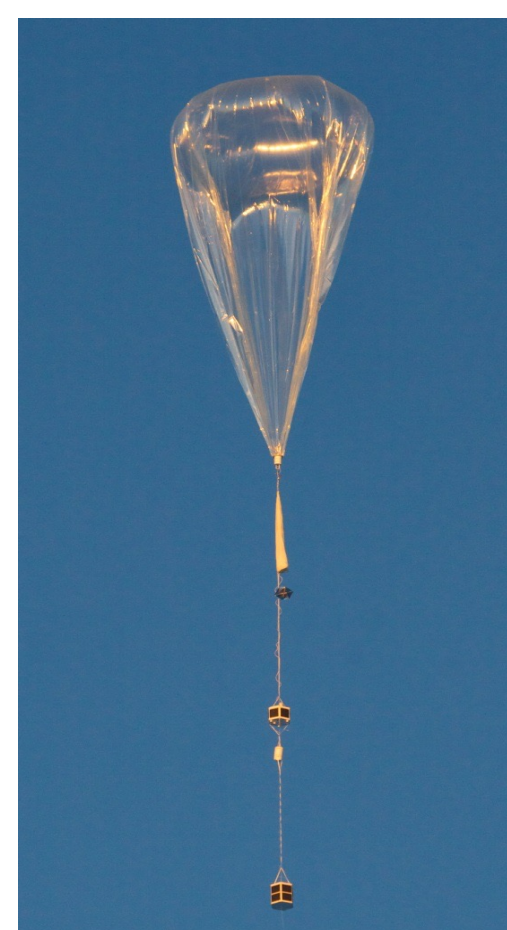
Spherical Helium Super Pressure Balloons, 11 and 13-m diameter, fly at 18 and 20 km altitude, respectively.
