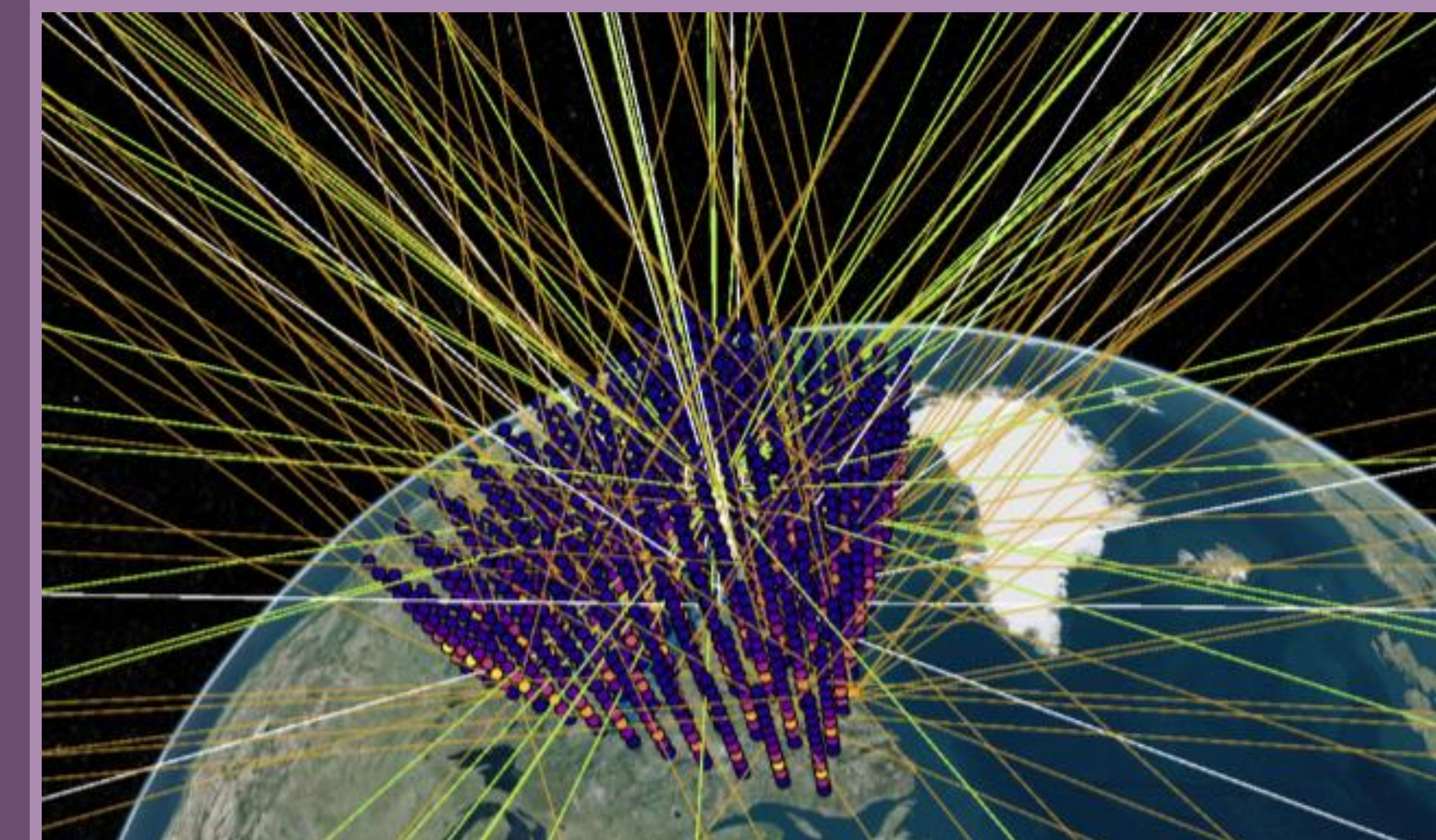
Figure X. Three-dimensional visualization of the simulated tomographic process using Cesium software. Figure produced by Brian Breitsch, software currently in use throughout project to assess program performance. White rays = ground-based, green rays = GNSS-RO, and orange rays = reflected.
