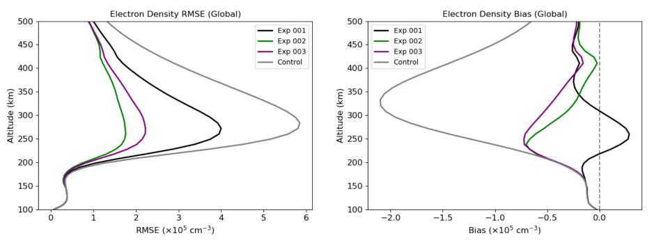
Going from ~20,000 occultations/day (Exp 003) to almost 30,000 occultations/day (Exp 002) leads to an additional ~8% reduction in global electron density errors at ~300 km.
